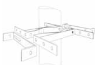
Mast bratchet dia 30-110 mm code xxxxx 1 pannel 2 pannel 90° 2 pannel opposite 180° 3 pannel 270°
