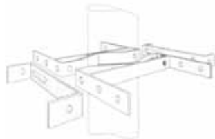
Mast bracket dia 30-110 mm code xxxxx 1 pannel 2 pannel 90° 2 pannel opposite 180° 3 pannel 270°
